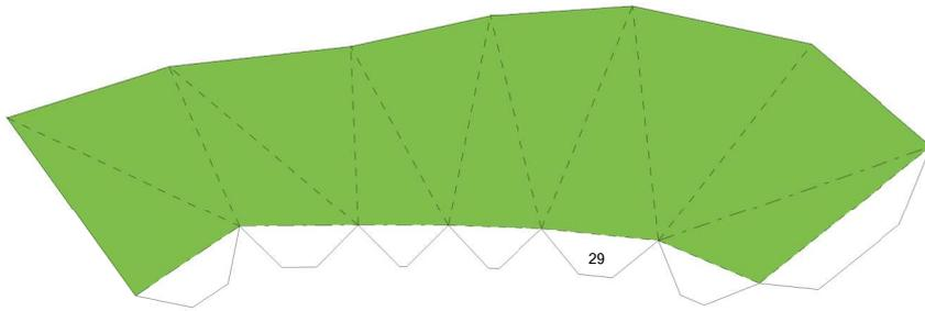
Close the model at the tail and glue piece 34 after it's closed. Also, keep in mind that it don't stand on it's own. You'll need some coins in the tail, just add some coins before closing untill it stands, and after closing, make the coins go to the tail by carefully moving the body. Don't forget to place the bone before counterweighting.
