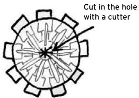
7. For the simplified engine, cut out the engine plate and make a hole in the middle. Roll the engine shaft around a toothpick, that the toothpick can comfortably rotate inside of it. Then glue the shaft into the hole, and align it from the line on it.
