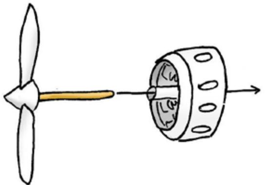
11. Glue the second shaft hub to the end. Make sure no glue gets between toothpick and shaft.
