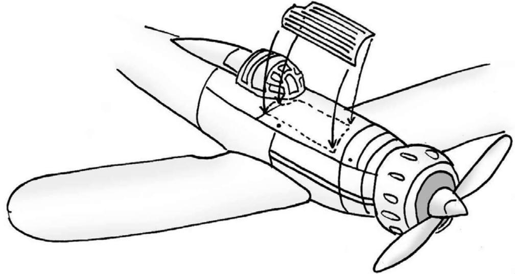
25. Bend down the front part of the fuselage bottom, then glue it across wings and fuselage
