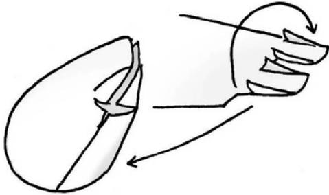
2. Glue together the fuselage parts, starting in the middle.
