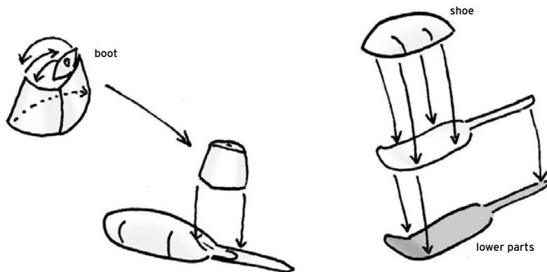
29. To build the ski shoes, rounden and glue the boot. Then glue together the lower parts, bend up both ends, glue the shoe on them, then the boot on the angle at the back of the shoe. The upper part must be parallel to the ski.
