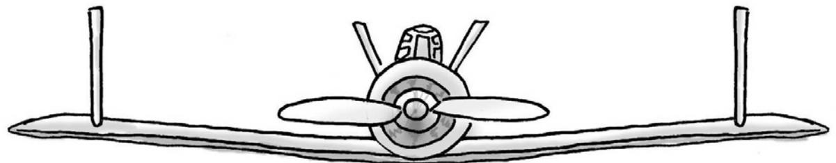
27. Glue the upper wing on the wing struts. Make sure to align the struts to sit on the round markings.
