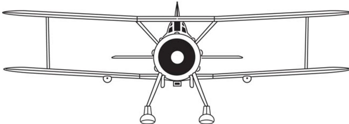
5. For the Propeller, first make a hole in the shaft hub. Then glue together spinner and blades. Glue the blades on the lines marked on the spinner.
