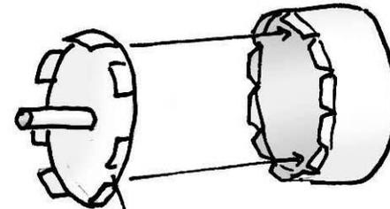
8. Build the main cowling part and glue the engine plate on the front end. Align the front end of the engine plate's flaps with the front of the cowling part.
