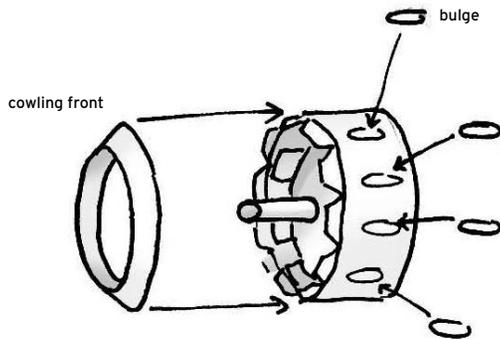
10. Push the Propeller through the shaft. **Don't glue!**
