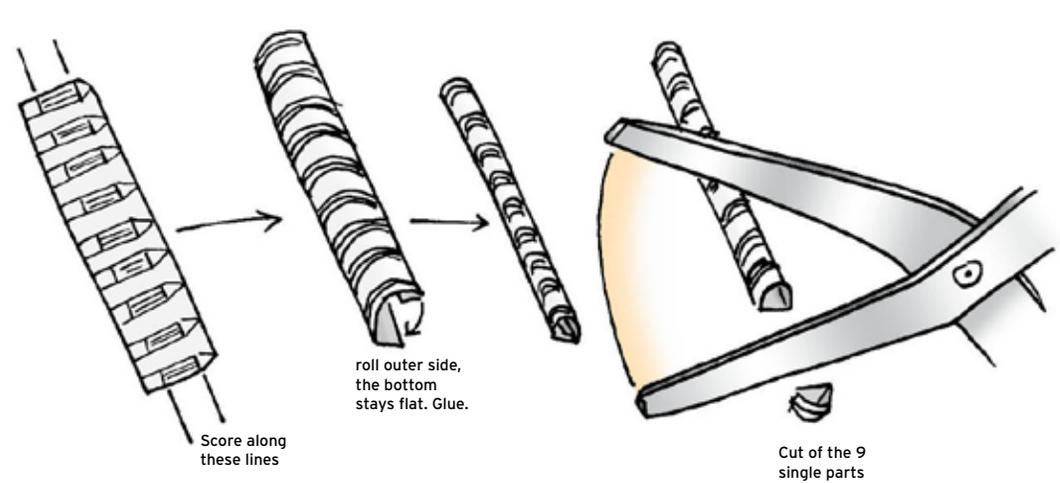
14. The part on the left side on the page appears smaller, but has the wider diameter. Glue these on the outer ring of the baseplate first.
