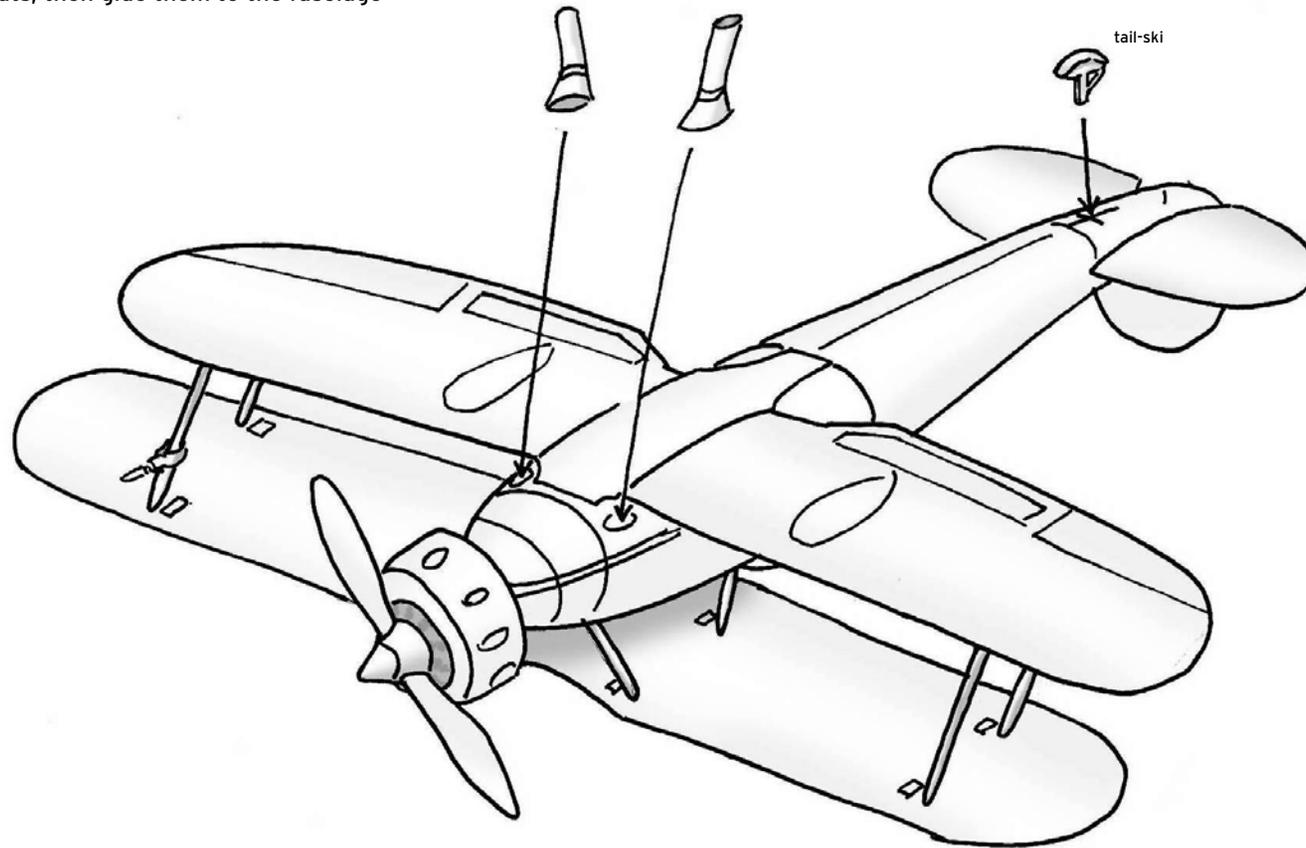
Glue together the two halves of both parts of the tail-ski, then bend the lower part to fit around the vertical part
